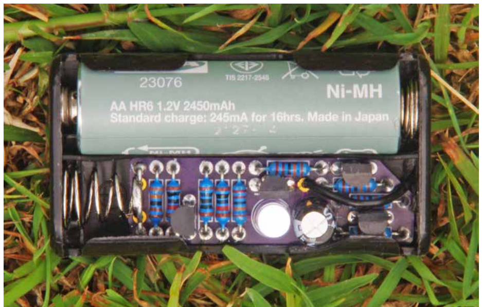
The circuit board takes the place of one of the batteries in the AA battery holder.
